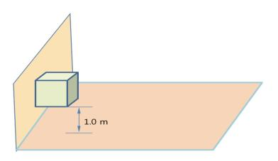
Figure 3 - Wall-mounted noise measurement location
