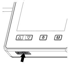
The unit has a slot for a memory card. The slot is only required for service purposes.
