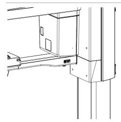
Figure 5: Emergency stop switch on the patient side
