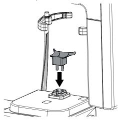
Inserting the positioning aid for panoramic images with hygienic protective cover (optional)
