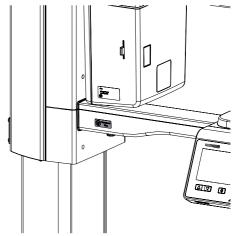
Figure 4: Emergency stop switch on the operator side
