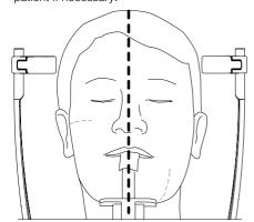
Align the head of the patient according to the Frankfurt horizontal plane with the aid of the X-ray positioning beam.
