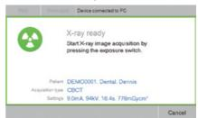
> Trigger the image by pressing and holding the button on the exposure switch until the acoustic signal stops and the control lamp goes out. The scanning times depend on the patient type, imaging program and image quality (see "13 Program parameters").
