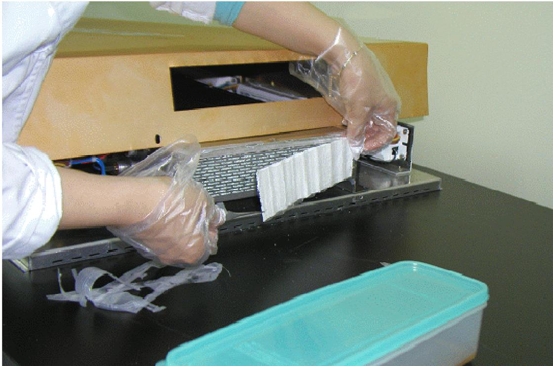
Figure 2). MDS filter attached at the exit of the Viruskiller
