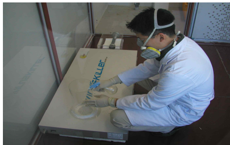
Figure 4. Atomizing injection of strain in inlet port of VirusKiller
