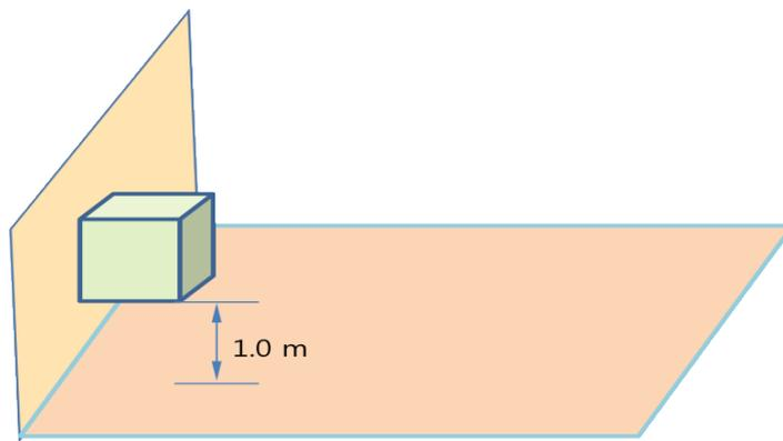
Figure 3 - Wall-mounted noise measurement location
