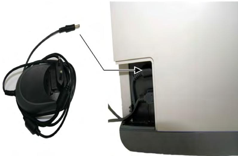
4. Connect the USB cable to the dedicated connector in the cable compartment, and route the cable as shown on the below image to secure the cable in its place:
