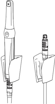
Whenever the camera is in the handpiece holder, it is switched off. When you remove the camera from the handpiece holder, it switches on automatically.
