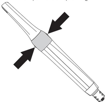
The camera switches to "Freeze" mode. The freeze frame will be displayed in the imaging program / transmitted to the monitor.
