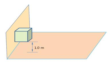
Figure 3 - Wall-mounted noise measurement location
