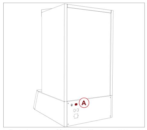
The sintering oven has an RS-232 interface (A) on the rear, which is used to save log files on a computer.
